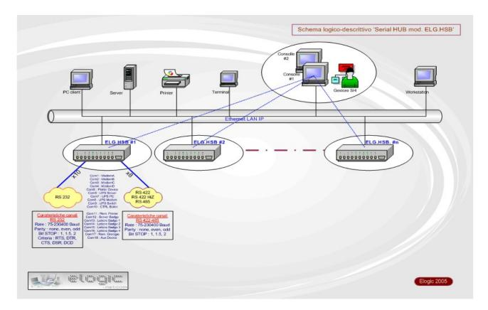
The serial HUB RCK02 is a device with two independent LAN channels (HSUB 1 and HSUB 2) that expands up to twenty serial interfaces.
